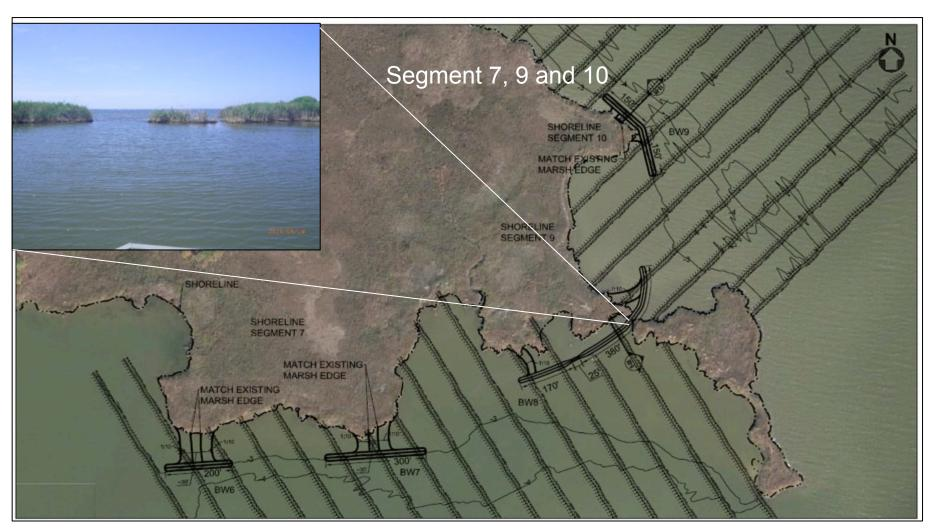
These alignments are considered headland control since they are placed sufficiently close to existing hard points extending seaward from the shoreline. The purpose of these structures is to protect these shoreline headlands which help shape the bay shoreline by wave diffraction.
